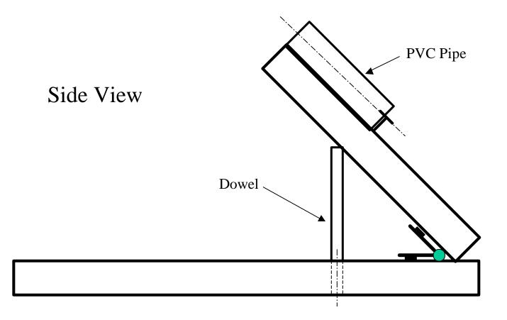
5. To build the "pusher" for the launcher, drill a 3/16" hole through the narrow edge of a 2"x<sup>1</sup>/2"x<sup>1</sup>/2" piece of bass wood or similar material. Attach springs, thumbtacks, bolt, nut, and wingnuts as shown:
