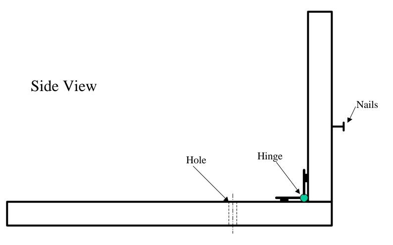
4. Cut a 4" long piece off of a ¼" diameter dowel. By inserting the dowel in the hole, you should be able to set the launcher at a stable angle. With tape or glue, attach a 4" long piece of PVC pipe to the center of the upper wood piece, from the tip to the nails.
