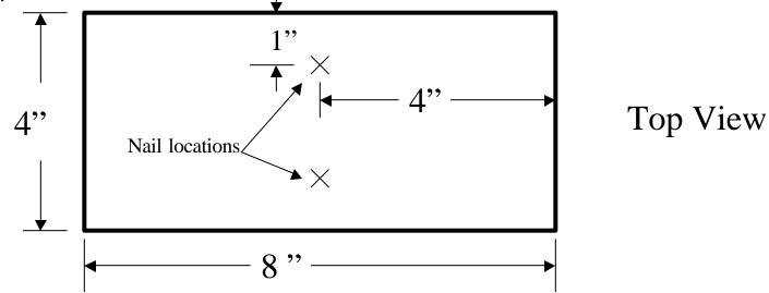
3. Attach the two boards together with a hinge so that they can open to a right angle, with nails and hole oriented as shown below. Pilot holes may be helpful for attaching the screws holding the hinge in place.
